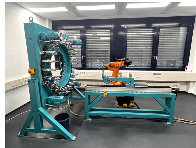
Medical-grade weaving for Alaxo nasal stents
